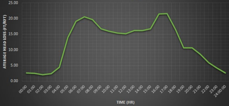
Ductile Iron (closed tank) Average Headloss vs Time
