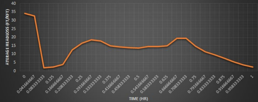
Ductile Iron Headloss Average (open tank) Headloss vs Time
