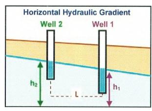
over the change in distance between the two monitoring wells or dh/dl.
