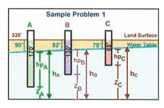
a. What is the hydraulic head (h) at each? (surface elevation - depth to water)
