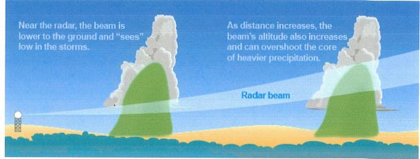
reflectivity is excellent for surveying the region around the radar to look for precipitation. However, remember the radar beam increases in elevation as distance increases from the radar. This is due, in part, to the elevation angle itself but is more because the earth's surface curves away from the beam.
