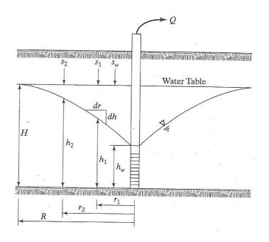
$$Q = \frac{\pi K (h_2^2 - h_1^2)}{\ln(r_2/r_1)}$$
