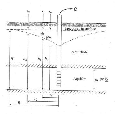
$$Q = \frac{2\pi T (h_2 - h_1)}{\ln(r_2/r_1)}$$
