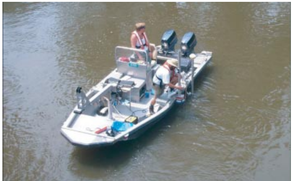
Fig. 1. Hydrographers measure stream flow using an Acoustic Doppler Current Profiler (ADCP) on the Kankakee River at Dunns Bridge, Indiana.
