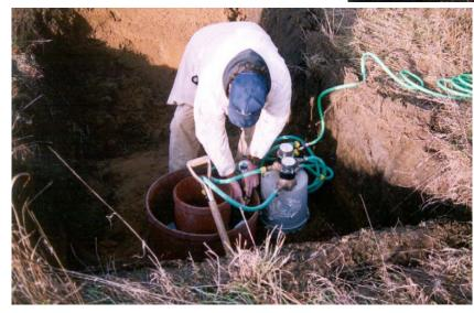
This test can be used for infiltration basins, on-land disposal of secondarily treated effluent or ponded storm water. The test can be run at various elevations in stratified soils by excavating shallow test pits.
