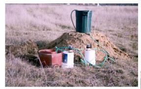
The double-ring infiltrometer test (ASTM D3385) is a field method to determine the infiltration rate of a fluid (wastewater or storm water) into soil on a planar surface. It is relatively simple and inexpensive and provides a direct infiltration rate, as opposed to the percolation test or the laboratory permeability test.
