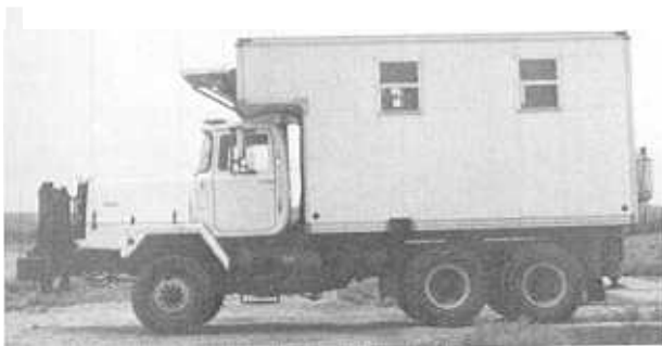
Figure 5-40.—Self-contained, truck-mounted, electrical cone-penetration apparatus.
