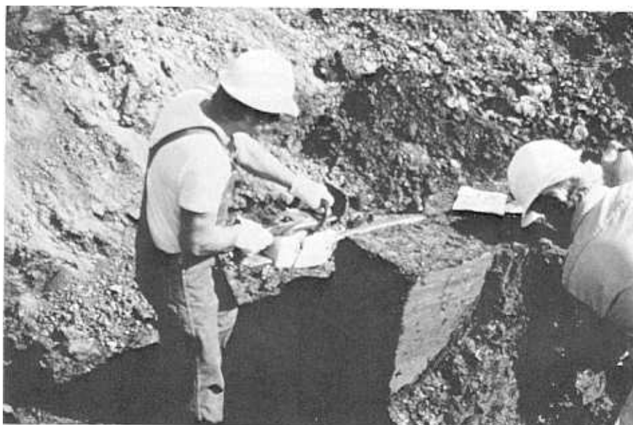
Figure 5-58.—Chain saw equipped with carbide-tipped blade being used to cut block sample.
