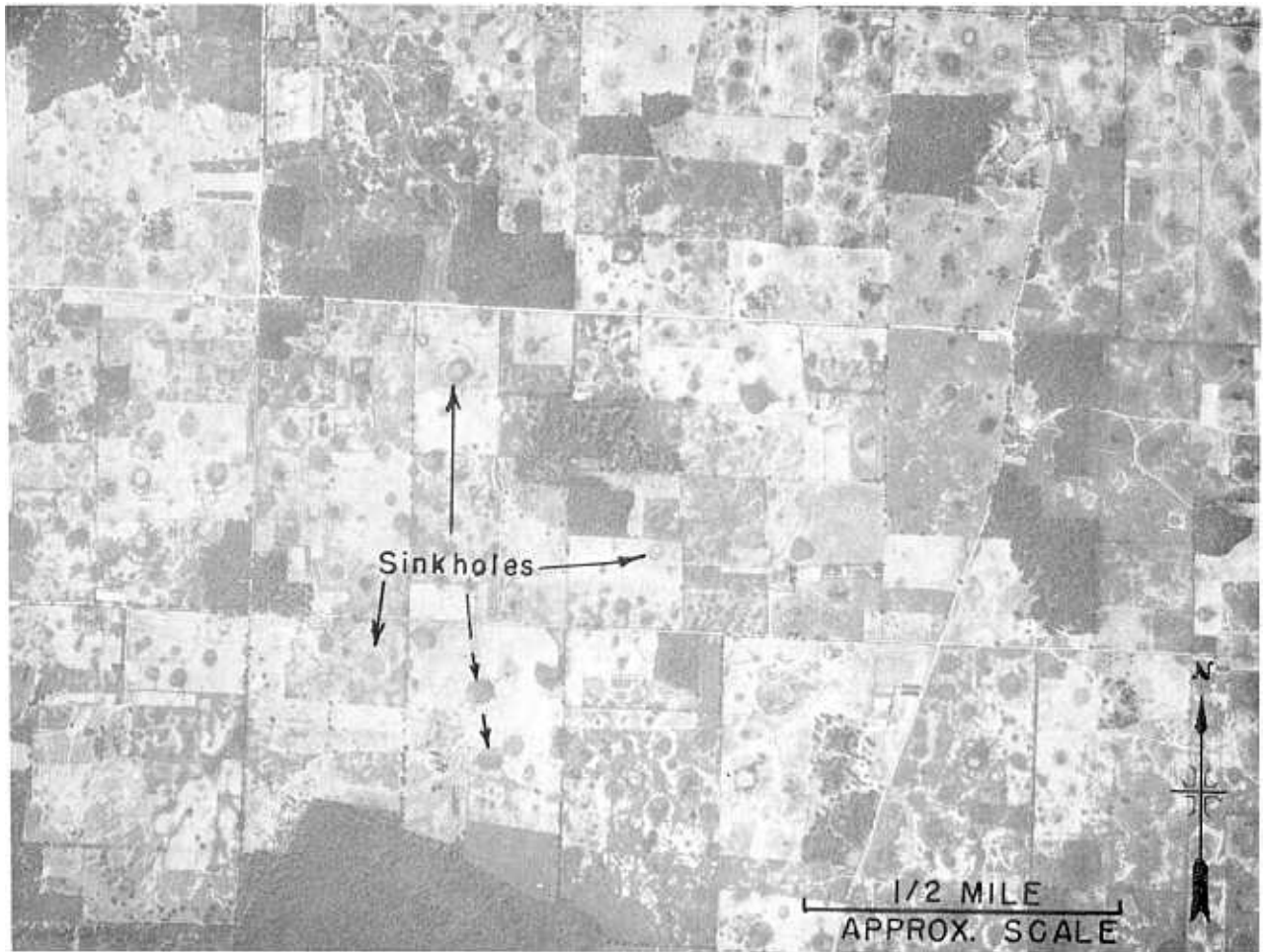
Figure 5-6.—Sinkhole plain indicating deep plastic soils over cavernous limestone, developed in humid climate. (U.S. Agricultural Stabilization and Conservation Service). PX-D-16264.
