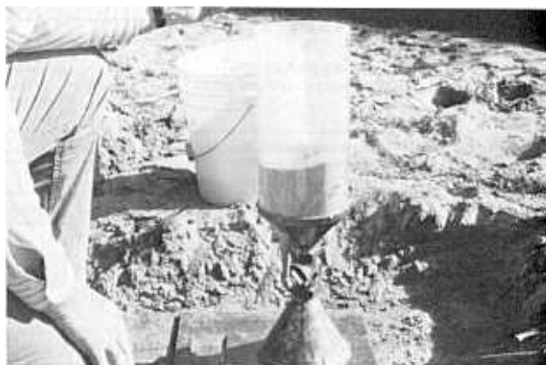
Figure 5-71.—Determining inplace unit weight by replacing soil with a sand of known unit weight.
