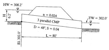
The invert elevation of the culvert at the outlet is  $(302.0 - 80 \times 0.04) = 298.8$  ft and the crown elevation at the outlet is (298.8 + 4.0) = 302.8 ft. The headloss through the culvert with outlet control is (308.2 - 302.8) = 5.4 ft. The discharge rate computed for both outlet and inlet controls are as follows:
